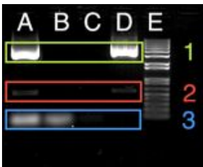
Figure 0.11: Agarose gel analysis for pDNA. At different stages during the purification process, fractions were collected and run in a 1% agarose gel containing ethidium bromide. UV microscopy was used to visualize the bands. Different features of the analysis are shown. The upper band (1) shows open circular form and the middle band (2) shows the supercoiled form of the amplified plasmid DNA in both the unpurified (A) and final purification (D) steps. The additional band (3) shown in the unpurified (A) step shows the degraded RNA impurity. This band is also present in the flow-through fraction (B) collected before washing the DNA, and a faint shadow of the band is seen in the flow-through fraction from the wash step (C). It is not present in the final purification step (D), indicating successful removal of the impurities.
